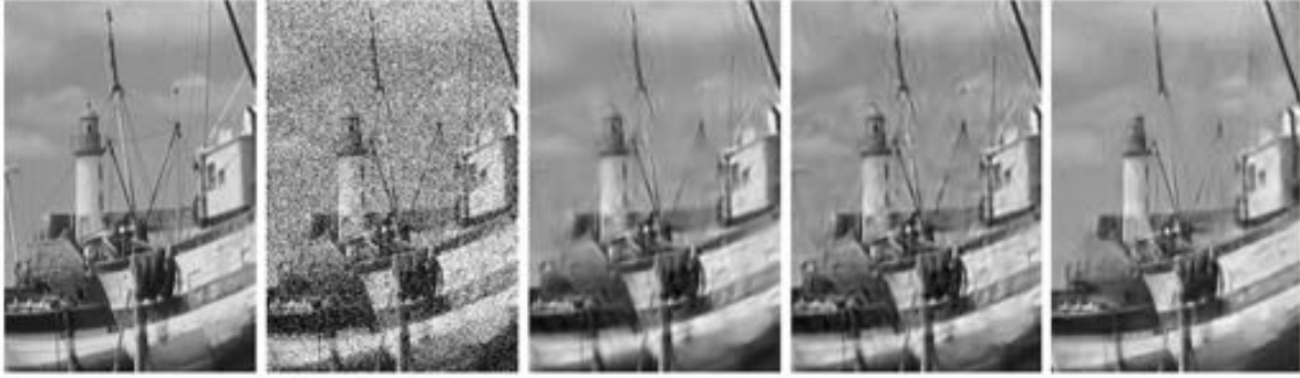
Figure 1: From left to right: original, noisy image ( \sigma = 50 ) ; Gaussian scale mixture by Bayesian least squares [23] (PSNR=26.3) ; fields of Gaussian scale mixtures [20], (PSNR = 27.0); and the proposed multi-scale DCT pyramid applied to BM3D (PSNR = 26.73). In spite of their excellent PSNR performance these methods suffer from severe ringing artefacts. Being inherently already multi-band, they cannot benefit from the conservative recombination proposed here.
