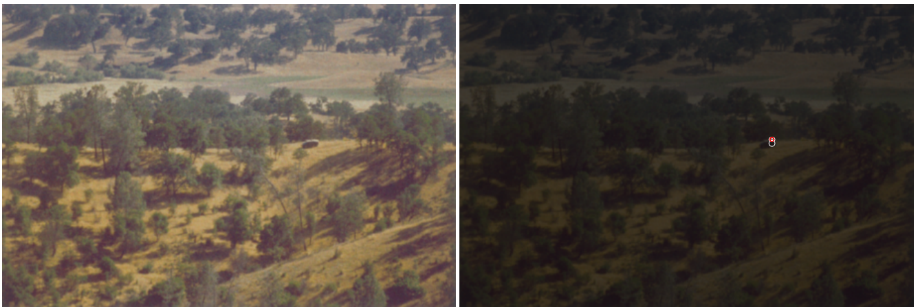
Fig. 9. Left: Input image, Right: detections with pixels . The method successfully detects a tank hidden in the landscape. This example is one of the examples provided by Itti et al. [6]
