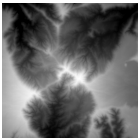
(a) A plausible evolution of the digital elevation model where 10% of the terrain has been removed by erosion.
