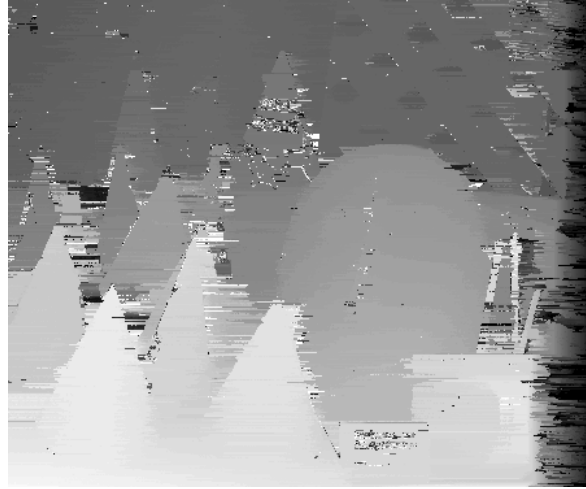
Figure 5.2 – Disparity map obtained on the Middlebury stereo pair Cones by minimizing the 1D energy (5.9) row by row. The streaking artifacts are due to the absence of regularity constraints in the vertical direction.
