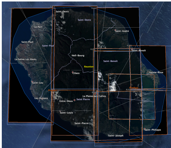
Figure 6.7 – Coverage of the Réunion island by Pléiades stereo images. Eight stereo pairs and one tri-stereo dataset were used. Each rectangle corresponds to a dataset. The largest image has dimensions of approximately 40\,000 \times 120\,000 pixels. Some clouds are visible in white. They correspond to the holes of the digital elevation model of figure 6.8. Copyright ©CNES 2011-15, distribution Airbus DS / Spot Image
