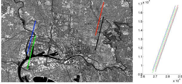
Fig. 1. The RPC functions allow to draw the epipolar curves for a pair of Pléiades images u and v (approx. 40\,000 \times 16\,000 pixels). The left image shows four epipolar curves plotted in the domain of image v . They correspond to four points located near the edges of the image u . The range of altitudes considered is h \in [-200, 3000] meters. The right image shows the same epipolar curves placed closer to facilitate the comparison.
