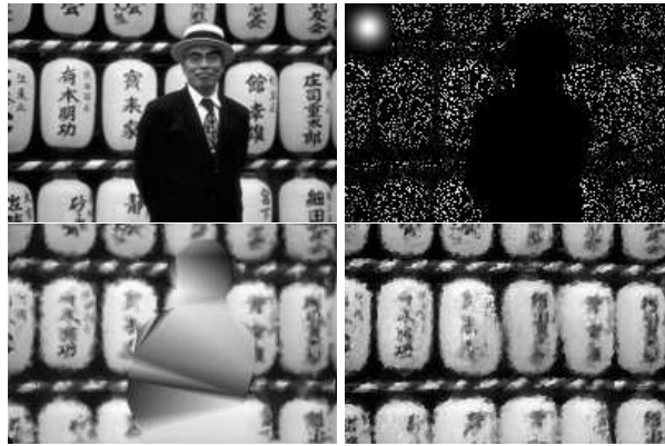
(a) Cylinders , 200 \times 113 . Inpainting a hole in a subsampled image with algorithm B . The algorithm makes no distinction between the hole and the sampled regions. The sampling density is 20% yielding a global sampling density of 14%.
