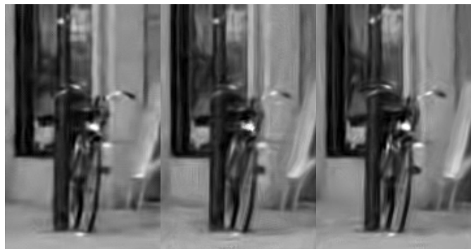
Fig. 1. Detail of the results obtained with BM4D-OF, VNLDCT and VNLB on the pedestrian sequence for a noise of standard deviation \sigma = 40 . The contrast has been linearly enhanced to make the differences between the methods more visible.
