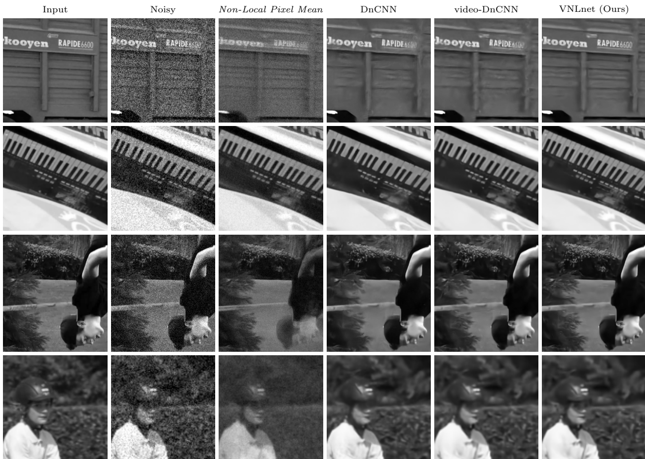
Fig. 5: Example of denoised result for Non-Local Pixel Mean , DnCNN, video-DnCNN (see Section 4.3) and VNLnet, for AGWN with \sigma = 20 . The four crops highlight the results on frames feature various kinds of motion. The videos are part of the DAVIS dataset. Non-Local Pixel Mean corresponds to the average of the output of the non-local patch search.
