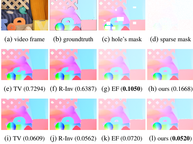
Fig. 3: Comparison of different motion completion algorithms in two different cases: inpainting of large holes (holes in white in image (c) and results shown in the 2nd row) and flow densification from a sparse set of ground truth matches (shown in image (d) and results in 3rd row). The methods used are TV [24], R-Inv [21], EpicFlow (EF) [22] and ours. For the EpicFlow we consider only the interpolation step and overwrite the result with the ground truth flow outside the inpainting mask. Numbers in parenthesis show the EPE for each result.
