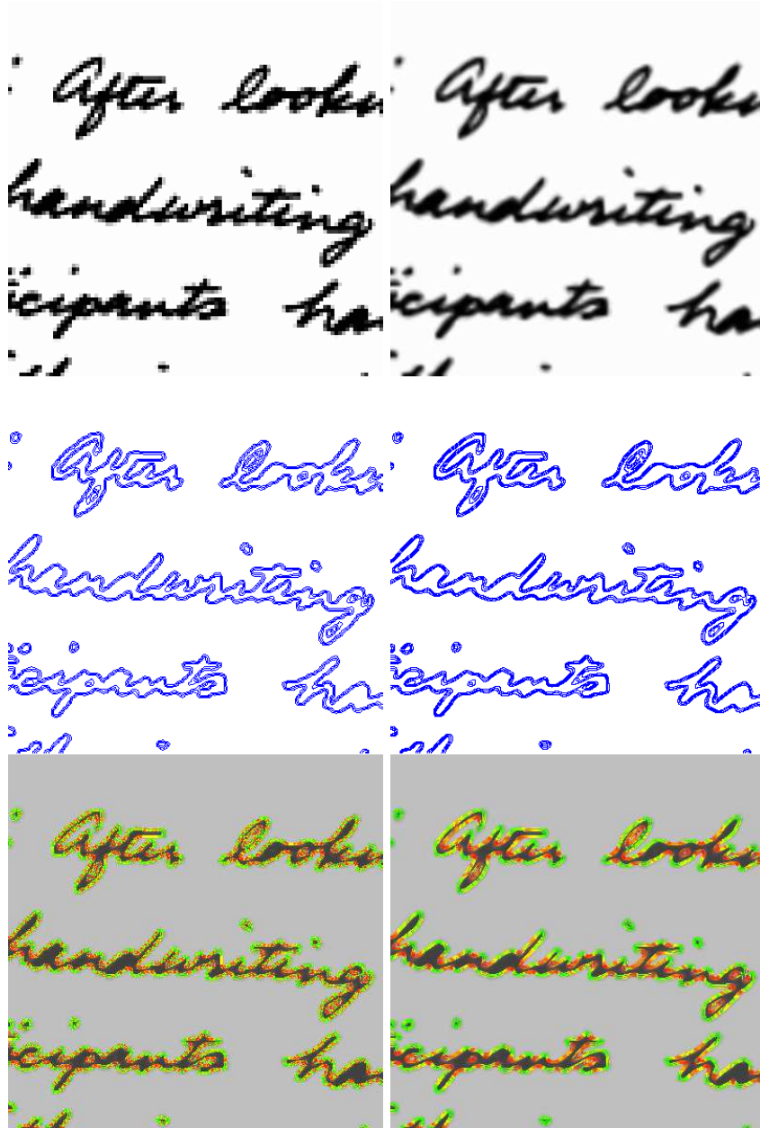
FIGURE 19. Left: original image, bilinear level lines and the curvature map before filtering. Right: smoothed image, affine smoothed level lines and curvature map after filtering.
