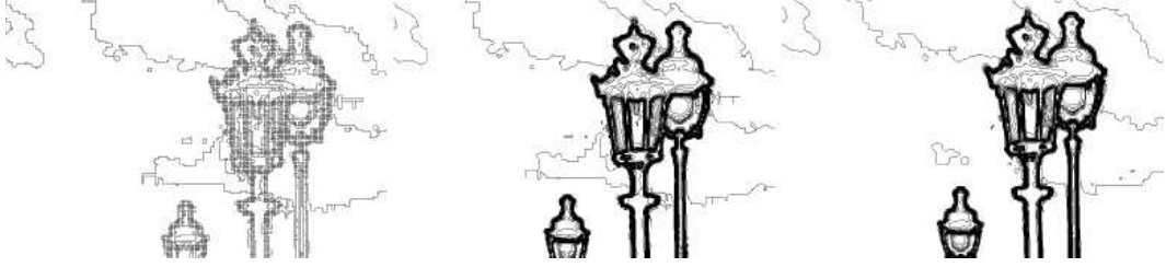
FIGURE 2. Left: level lines from a digital image (zero-order interpolation). The quantization step for the gray levels is 10, starting from 10. The pixelization effect creates artificial T-junctions, and do not allow to compute useful features such as inflexion points or curvature extrema. Middle: level lines from the piecewise bilinear interpolated image. The quantization step for the gray levels is 10, starting from 10. Pixelization effect has been reduced, but some pixelized regions can still be seen. Right: level lines from the piecewise bilinear interpolated image, with a gray level quantization step of 10, starting at gray level 0:5. These level lines do not suffer from pixelization effects.
