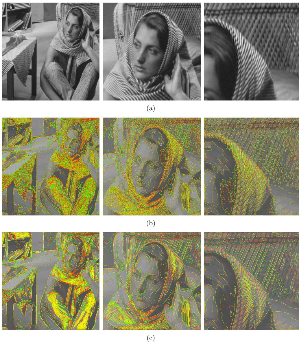
FIGURE 4. Image curvature microscope. (a) the original image, 2X zoom and 4X zoom of the up-right corner; (b) curvature map computed on the original level lines with a quantization step s = 36 ; (c) curvature map computed on shortened level lines. The left column permits to observe the curvature densities. A zoom is necessary to observe the single curvatures. The middle column and right column focus more and more on shape and texture details.
