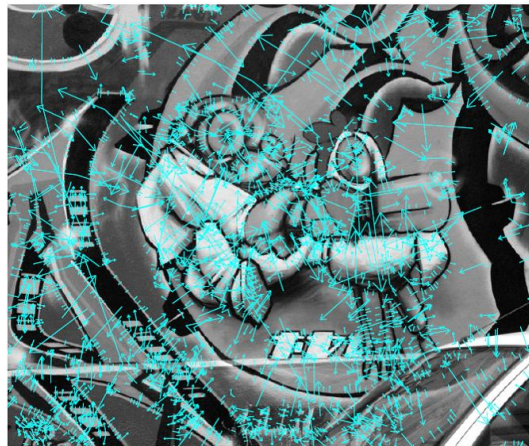
Figure 3: SIFT key points. The arrow starting point, length and the orientation signify respectively the key point position, scale, and dominant orientation. These features are claimed to be covariant to any image similarity.
