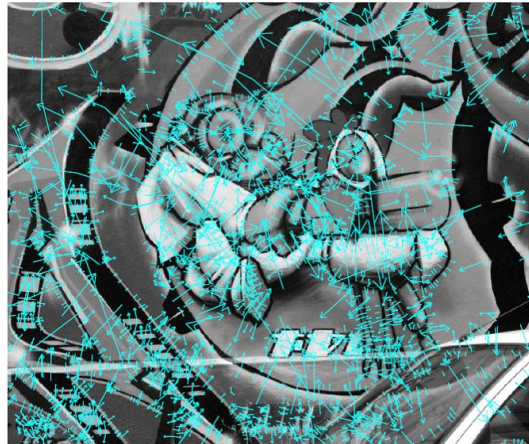
Figure 11: SIFT key points. The arrow starting point, length and the orientation signify respectively the key point position, scale, and dominant orientation. These features are claimed to be covariant to any image similarity.
