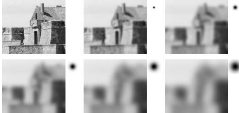
Figure 4: Convolution with Gaussian kernels (heat equation). Displayed from top-left to bottom-right are the original image and the results of convolutions with Gaussians of increasing variance. A grey level representation of the convolution kernel is put on the right of each convolved image to give an idea of the size of the involved neighborhood.
