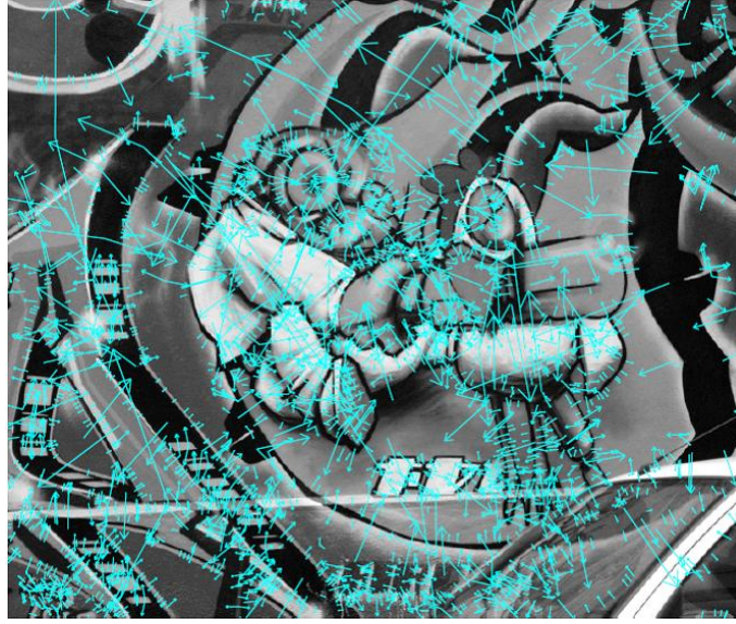
Figure 8: SIFT key points. The arrow starting point, length and the orientation signify respectively the key point position, scale, and dominant orientation. These features are covariant to any image similarity.
