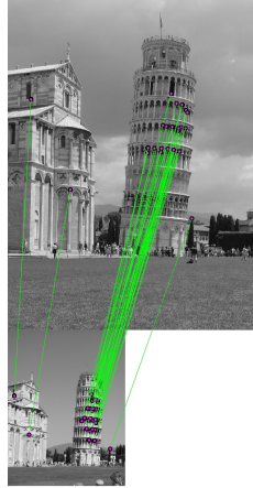
Figure 1: A result of the SIFT method, using an outliers elimination method [37]. Pairs of matching points are connected by segments.
