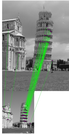
Figure 5: A result of the SIFT method, using an outliers elimination method [37]. Pairs of matching points are connected by segments.
