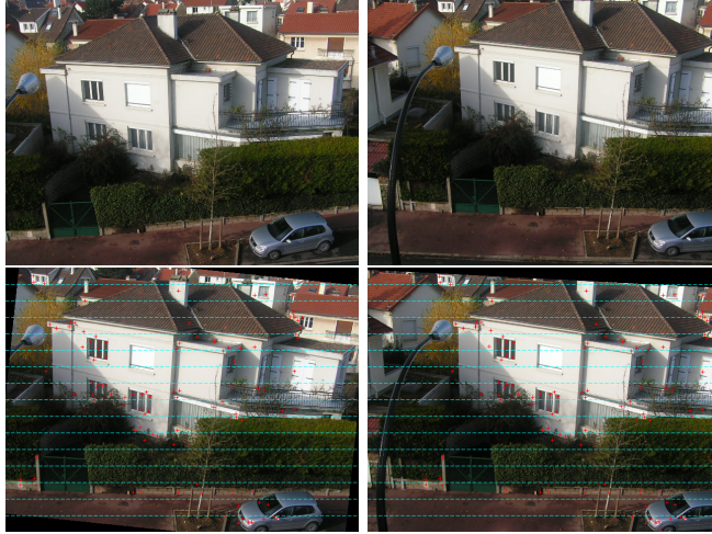
Figure 6: Rectification example. Top: a pair of original images. Bottom: the rectified images, with some epipolar lines and matching points marked as crosses
