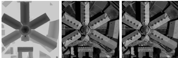
Figure 7: Synthetic image pair. Left: the disparity ground truth. The background has uniform disparity while the building has a sloped roof. Center and right: image pair.
