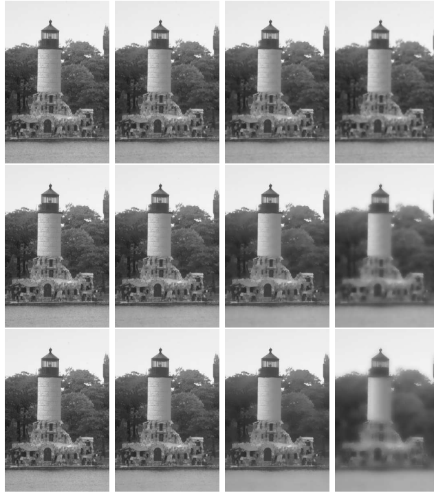
Figure 1.3: Several applications of the Bilateral filter for increasing values of parameters \rho and h . The parameter \rho increases from top to bottom taking values \{2, 5, 10\} and h increases from left to right taking value \{5, 10, 25, 100\} .
