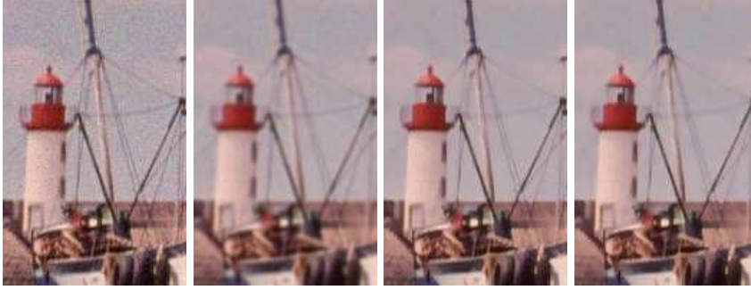
Figure 1.2: From left to right: noise image, Gaussian convolution, neighborhood filter and Bilateral filter. The neighborhood and Bilateral filters avoid the excessive blurring caused by a Gaussian convolution and preserve all contrasted edges in the image.
