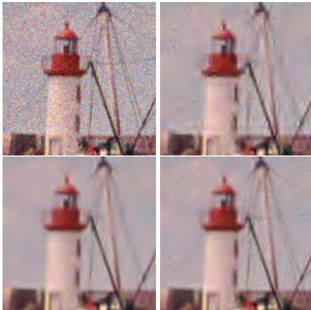
FIG. 4. Denoising experiment on a natural image. From left to right and from top to bottom: noisy image (standard deviation \sigma = 20 ), the wavelet hard thresholding (HWT, \mu = 3\sigma ), translation invariant hard wavelet thresholding (TIHWT, \mu = 3\sigma ) and the DCT empirical Wiener filter ( W = 15 \times 15 pixels, \mu = \sigma/2 ). Parameters have been set for each algorithm in such a way the removed energy is similar to the added noise energy, \sigma^2 , getting the best result in terms of euclidean distance to the original image.
