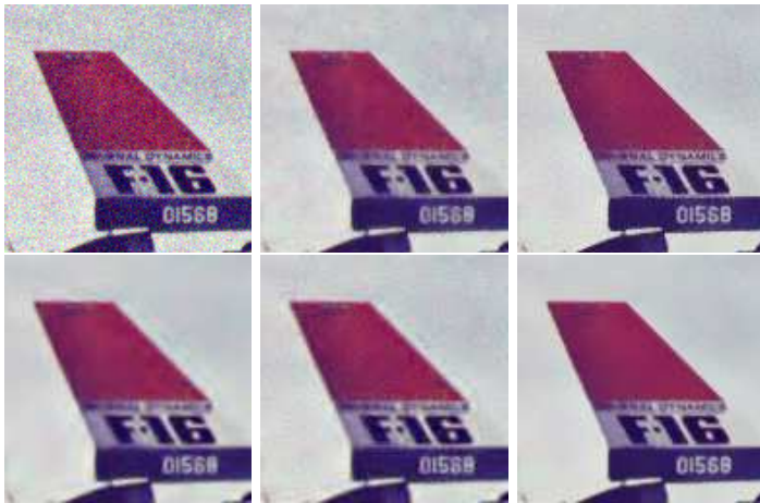
FIG. 15. Denoising experience on a natural image. From left to right and from top to bottom: noisy image (standard deviation 35), total variation, neighborhood filter, translation invariant hard thresholding (TIHWT), empirical Wiener and NL-means.
