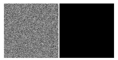
**Square:** The square is masked by noise and is not detected by LSD. But the square can be detected if the image is analyzed at a different scale by Gaussian sub-sampling.
