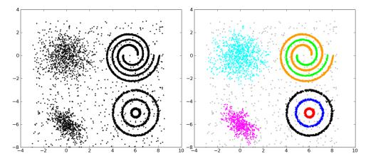
The algorithm depends on a notion of distance between points. With it, the Minimum Spanning Tree (MST) is computed (that is, an incomplete graph joining all points with the smallest sum of distances along its edges). A sub-graph of the MST will be considered meaningful when all the distances on the edges are too short to have arisen by random points with uniform distribution.
