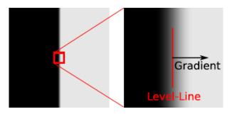
The algorithm starts by computing the level-line angle at each pixel to produce a *level-line field*. Then, this field is segmented into connected regions of pixels that share the same level-line angle up to a certain tolerance  $\tau$ . These connected regions are called *line support regions*:
