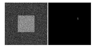
**Square-subsampling:** When a Gaussian sub-sampling is applied to the previous image, the noise is partially removed and the expected line segments are detected.
