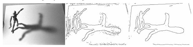
None of the two results are satisfactory. On the first one we get a detailed analysis of the mannequin, but the shadow produces a noisy result. On the other hand, when a larger scale is used the shadow is better resolved but at the price of missing the details on the mannequin. The detection threshold didn't perform a good job either as the spurious detections show.
