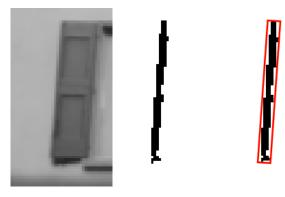
Each rectangle is subject to a validation procedure. The pixels in the rectangle whose level-line angle corresponds to the angle of the rectangle up to a tolerance  $\tau$  are called *aligned points*. The total number of pixels in the rectangle, n, and its number of *aligned points*, k, are counted and used to validate or not the rectangle as a detected *line segment*.
