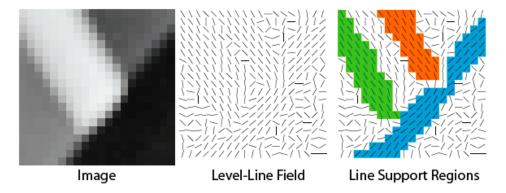
Each *line support region* (a set of pixels) is a candidate for a *line segment*. But the corresponding geometrical object (a rectangle in this case) must be associated with it. The principal inertial axis of the *line support region* is used as main rectangle direction; the size of the rectangle is chosen to cover the full region:
