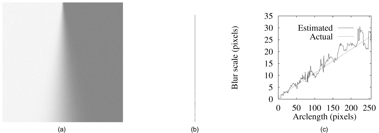
Fig. 7. Testing the local scale control algorithm on a synthetic image. (a) The blur grade is linear, ranging from \sigma_b = 1 pixel to \sigma_b = 26.6 pixels. The contrast of the edge and the amplitude of the added Gaussian noise are fixed. Parameters (see Section 4): A = B = 85 gray levels, \sigma_n \in [1, 26.6] pixels, s_n = 1.6 gray levels. (b) Detected edge. (c) Estimated vs. actual blur scale along edge.
