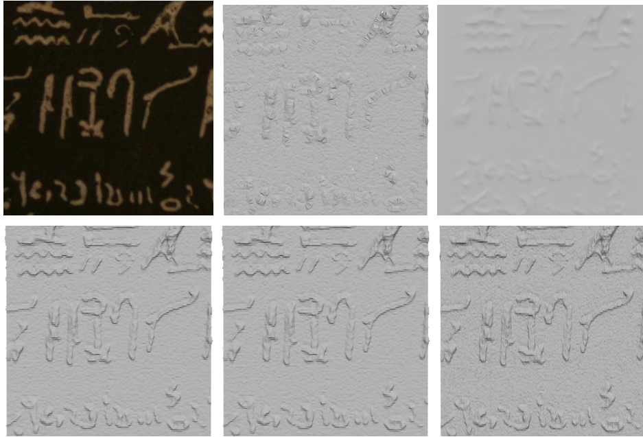
Figure 18: Comparison of the Rosette reconstruction (Picture (a)) using Ball Pivoting Algorithm (b), Poisson Reconstruction (c), RIMLS (d), APSS (e), and scale space meshing (f). APSS and RIMLS yield results that are really close to ours, yet both methods need an isosurface extraction done with the marching cubes, which creates strong artefacts (see a closeup Fig 19). Besides, RIMLS and APSS meshes contain around 268500 vertices whereas the scale space mesh contains 132203 vertices. Notice also that APSS and RIMLS introduce some denoising (visible especially in the nearly flat parts). Scale space meshing is the only method that preserves exactly the input data.
