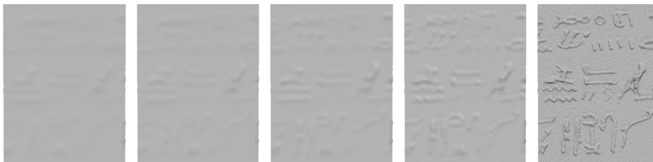
Figure 16: Back-projecting the mesh of a single scan of a fine-scale object (engravings are around 0.1mm deep). From left to right: mesh built after 4 scale space iterations; back-projection to levels 3, 2, 1 and 0 (final mesh).
