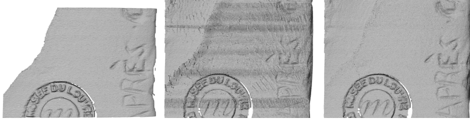
Figure 32: Comparison of the rendering of a single scan (ground truth) and the merging of all scans that overlap in the same region (Left: ground truth, middle: joint mesh of all scans without merging, right: joint mesh with merging).
