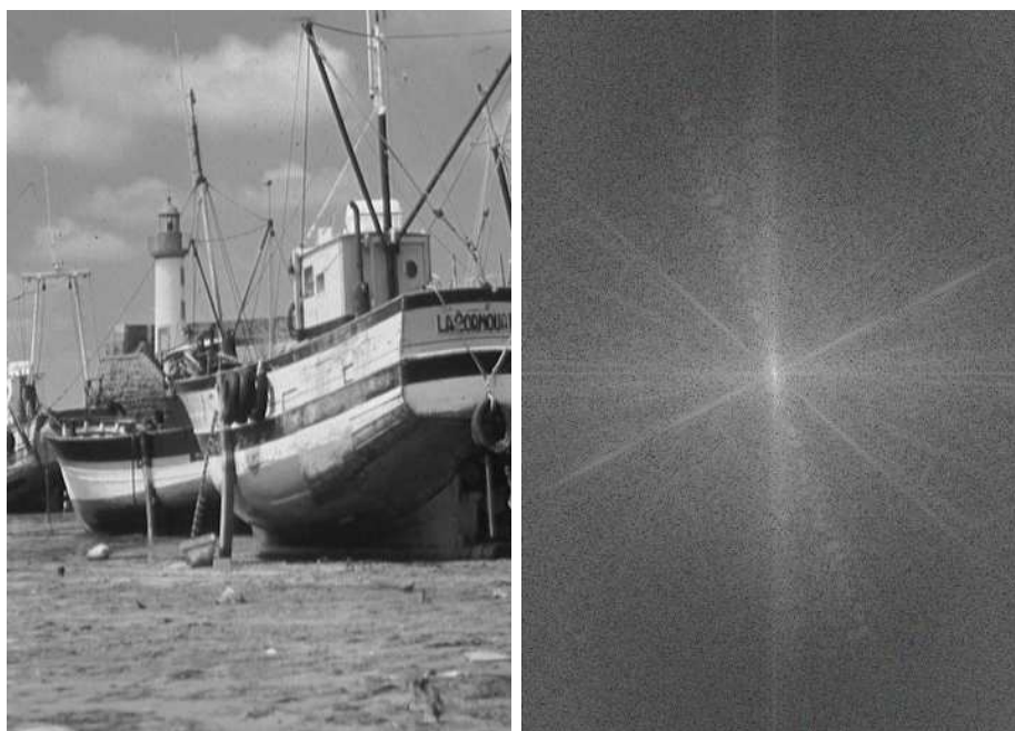
Figure 4: Acquired image (snapshot), the (log) modulus its Fourier transform .
