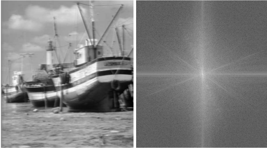
Figure 29: On the left : the acquired image for v = 1 , using the optimized code for Gaussian distributed motion with \sigma = 1 . On the right its Fourier transform (on a logarithmic scale).
