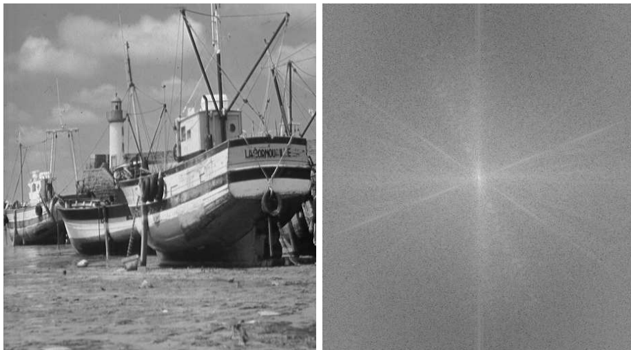
Figure 33: On the left : the acquired image for v = 0 , using the optimized code for Gaussian distributed motions with \sigma = 1 . On the right its Fourier transform (on a logarithmic scale).
