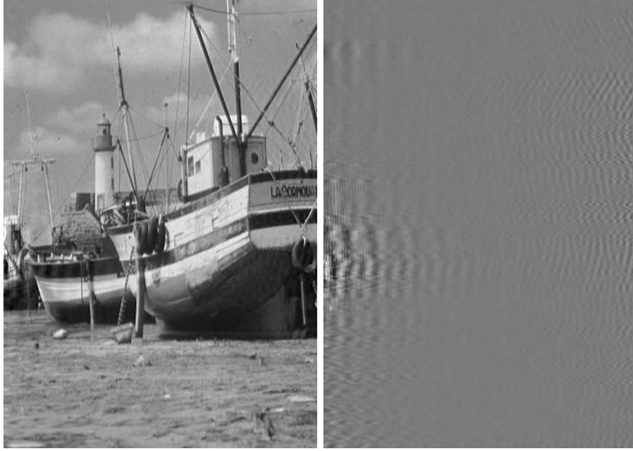
Figure 9: Restored image from the random code ( RMSE = 2.09 , RMSE_{CI} = 2.09 ), and the residual noise (contrast adjusted to [0, 255] ). Notice the boundary effects, which depend on the blur support. In practice if the image is large enough this should be negligible.
