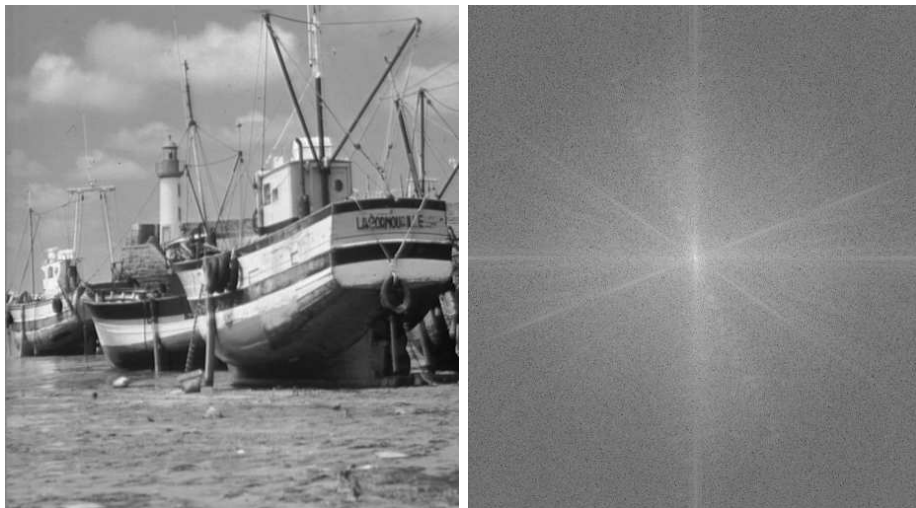
Figure 31: Acquired image for v = 0.25 , using the optimized code for Gaussian distributed motions with \sigma = 1 . On the right its Fourier transform (on a logarithmic scale).
