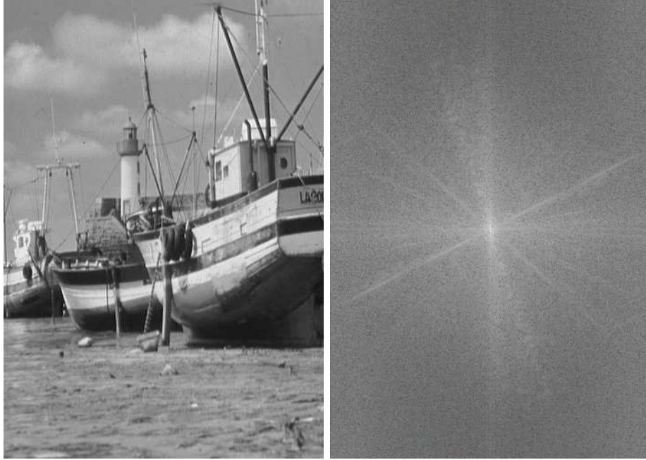
Figure 10: Acquired image with the sinc code and the (log) modulus of its Fourier transform. For a band limited image, the convolution a small enough sinc function is equivalent to a convolution against a dirac. This explains that almost no blur can be seen.
