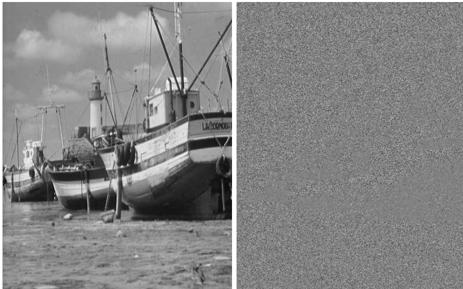
Figure 34: On the left : the restored image for v = 0 , using the optimized code for Gaussian distributed motion with \sigma = 1 , ( RMSE = 0.1897, RMSE_{CI} = 0.4319 ). On the right : the noise (rescaled on [0, 255] )
