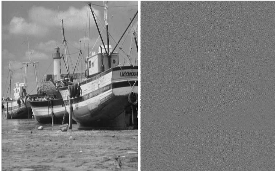
Figure 32: On the left : the restored image for v = 0.25 , using the optimized code for Gaussian distributed motions with \sigma = 1 , ( RMSE = 1.6600, RMSE_{CI} = 1.2572 ). On the right : the noise (rescaled on [0, 255] ).
