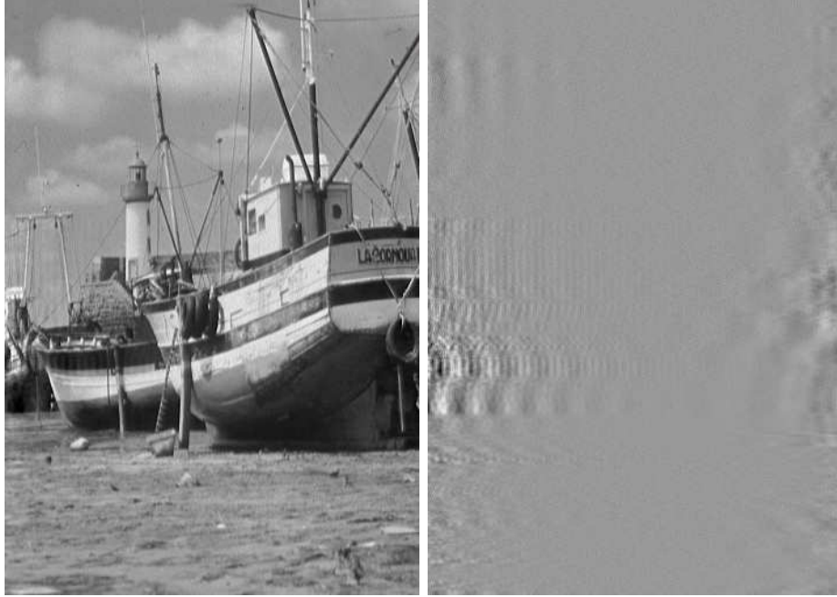
Figure 7: Restored image using the Raskar’s code ( RMSE = 2.30 , RMSE^{CI} = 2.32 ), and the residual noise (contrast adjusted to [0, 255] ). Notice the boundary effects which depend on the blur support. In practice if the image is big enough this should be negligible.
