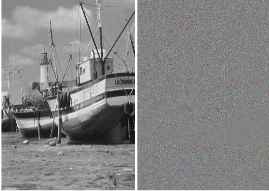
Figure 11: Restored image using the sinc code ( RMSE = 1.42 , RMSE^{CI} = 2.32 ), and the residual noise (contrast adjusted to [0, 255] ). Despite the deconvolution the noise remains almost a white noise since the Fourier transform of the sinc code is nearly constant.
