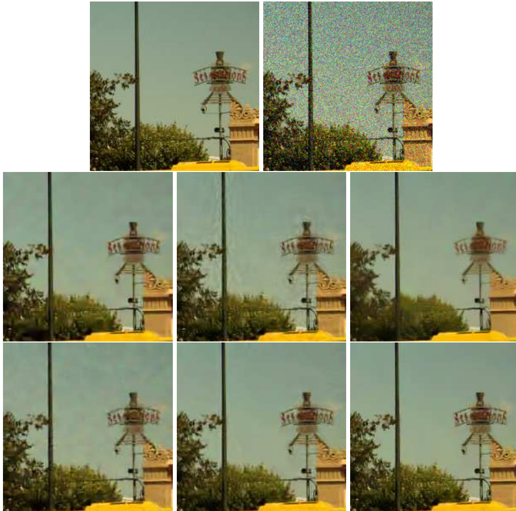
Figure 18: Comparison of visual quality. The noisy image was obtained adding a Gaussian white noise of standard deviation 30. From top to bottom and left to right: original, noisy, DCT sliding window, BLS-GSM, NL-means, K-SVD, BM3D and Non-local Bayes.
