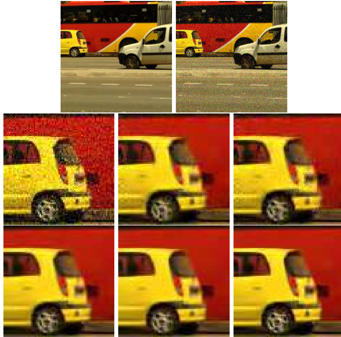
Figure 6: Top: original and noisy images with an additive Gaussian white noise of standard deviation 25. Below, from top to bottom and left to right: crop of denoised images by sliding DCT thresholding filter and incrementally adding use of a Y_oU_oV_o colour system, uniform aggregation, variance based aggregation and iteration with the “oracle” given by the first step. The corresponding PSNR are 26.85, 27.33, 30.65, 30.73, 31.25.
