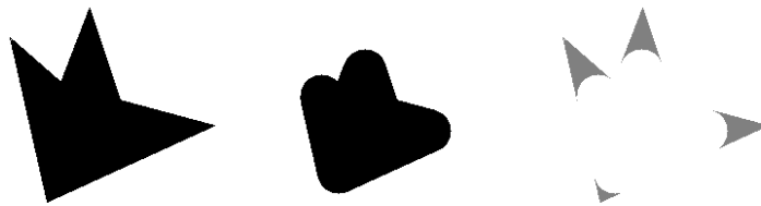
Figure 15.3: Opening of a set as curvature threshold from above. Left to right: A set X ; its opening by a ball of radius 20; the difference set. This opening transforms X into the union of all balls of radius 20 contained in it. The resulting operation can be understood as a threshold from above of the curvature of the set boundary.
