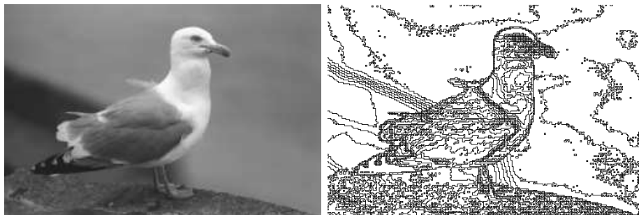
Figure 17.2: Level lines as a complete representation of the shapes present in an image. All level lines of the image of a sea bird for levels that are multiples of 12 are displayed. Notice that we do not need a previous smoothing to visualize the shape structures in an image: It is sufficient to quantize the displayed levels.
