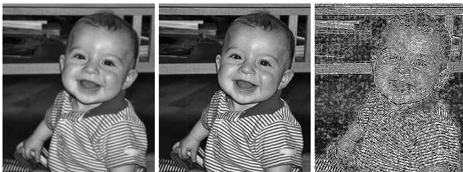
Figure I.7: Kovasznay–Joseph–Gabor deblurring. Left to right: original image; three iterations of the algorithm; ten iterations of the algorithm.
