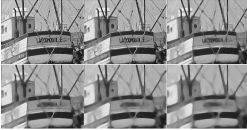
Figure 19.4: Curvature motion finite difference scheme applied on each level set separately, at scales 1, 2, 3, 4, 5. The processed image is then reconstructed by the threshold superposition principle. In contrast with the same scheme directly applied on the image, this scheme yields a fully contrast invariant smoothing. However, a comparison with Figure 19.3 shows that the resulting images are very close to each other. This shows that the contrast invariance is almost achieved when applying the finite difference scheme directly on a good quality image. As we shall see in Figure 19.6, if the initial image is noisy, the difference between both methods can be huge.
