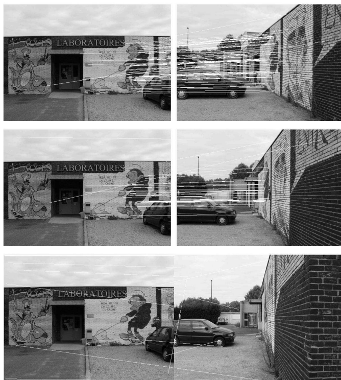
Figure 8.10: A-SIFT on an outdoor scene. From top to bottom: tilt distortion t between the two images are respectively t \approx 3.8, 5.6, 8 ; the number of matches are respectively 71 (4 false), 33 (4 false), 10 (all false).
