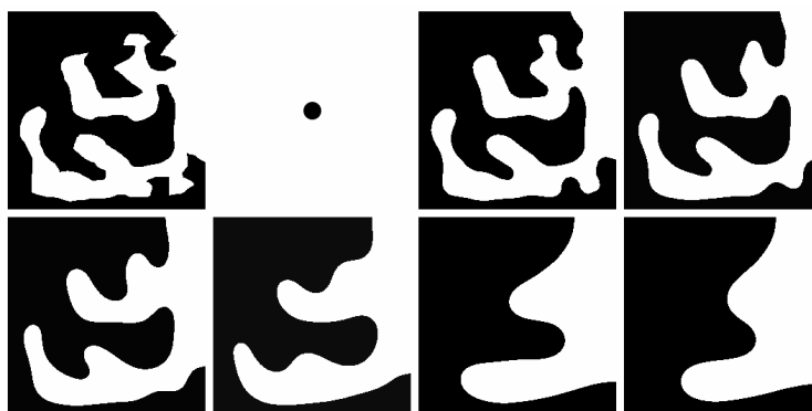
Figure 26.1: Scale-space based on iterations of the median filter. From left to right and top to bottom: original shape, size of the disk used for the median filter, and the results of applying the iterated median filter for an increasing number of iterations.
