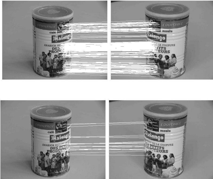
Figure 10.20: Image matching: can. Transition tilt \tau \in [2.3, \infty] . A-SIFT (shown), SIFT, Harris-Affine, Hessian-Affine, MSER+Corr and MSER+SIFT (shown) find respectively 287, 0, 6, 3, 12 and 22 correct matches. A-SIFT is implemented with K = 2 , which means that K = 3 doesn't work
