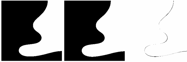
Figure 26.2: Comparing an iterated median filter with a curvature motion. Numerically, the iterated median filter and the curvature motion must be very close, at least when the curvatures of the level lines are not too small. Indeed, the iterated median filter converges towards the curvature motion. Left: the initial shape of Figure 26.1 has been smoothed by a finite difference scheme of the curvature motion; middle: smoothing with a median filter at the same scale; right: difference between left and middle images. The difference is no greater than the width of one pixel. To have a rigorous comparison, scales have been calibrated by ensuring that for both schemes and all r a circle with radius r vanishes at scale r
