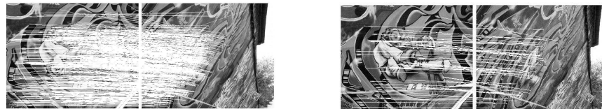
Figure 10.14: Image matching between Graffiti 1 and Graffiti 6. Transition tilt: \tau \approx 3.2 . From top to bottom, left to right: A-SIFT, SIFT, Harris-Affine, Hessian-Affine, MSER+Corr and MSER+SIFT find respectively 721, 0, 3, 1, 50 and 70 correct matches. A-SIFT is implemented with K = 3 . Results shown: A-SIFT and MSER+SIFT
