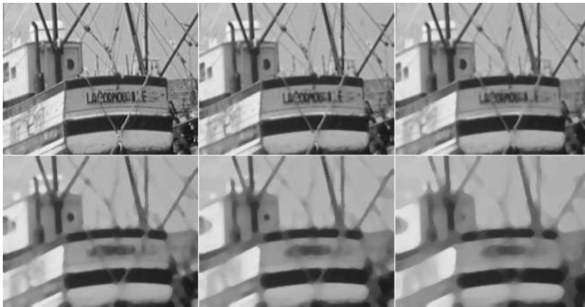
Figure 19.5: Iterated median filter with normalized scales 1, 2, 3, 4, 5. The scale normalization permits to compare very different schemes on the same images. Compare with Figure 19.4. The striking similarity of the results anticipates Theorem 20.7, according to which the application of the median filter is equivalent to a mean curvature motion.
