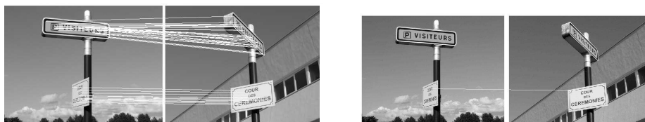
Figure 10.16: Image matching: road signs. Transition tilt \tau \approx 2.6 . A-SIFT (shown), SIFT, Harris-Affine, Hessian-Affine, MSER+Corr and MSER+SIFT (shown) find respectively 50, 0, 0, 0, 0 and 1 correct matches. A-SIFT is implemented with K = 3 .
