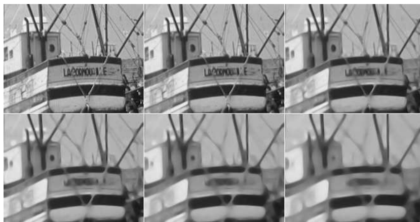
Figure 19.3: Curvature motion finite difference scheme and scale calibration. Image filtered by curvature motion at scales 1, 2, 3, 4, 5. In order to give a sound numerical meaning to the scale, a calibration of the numerical scales (number of iterations) is made in such a way that a disk with radius t shrinks to a point at scale t .
