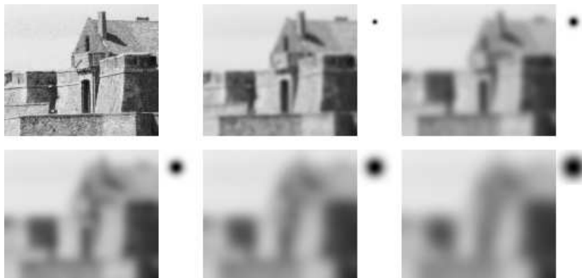
Figure 2.3: Convolution with Gaussian kernels (heat equation). Displayed from top-left to bottom-right are the original image and the results of convolutions with Gaussians of increasing variance. A grey level representation of the convolution kernel is put on the right of each convolved image to give an idea of the size of the involved neighborhood.
