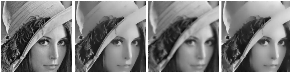
Figure I.14: Diffusion models II. Left to right: original image; Perona–Malik equation 1987, creating blurry parts separated by sharp edges; Carmona, Zhong 1998 which actually blurs the whole image: diffusion along the least eigenvector of D^2u ; Sochen, Kimmel, Malladi 1998: minimization of the image graph area. This last equation has effects similar to the Perona-Malik model.
