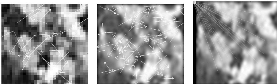
Figure 5.6: Scale invariance of SIFT, an illustration of Theorem 5.5. Left: a very small digital image \mathbf{u} with its 28 key points. For the conventions to represent key points and matches, see the comments in Fig. 5.4. Middle: this image is over sampled by a 32 factor to \mathbf{v} = \mathbf{S}_{\frac{1}{32}} I \mathbf{u} . It has 86 key points. Right: 22 matches found between \mathbf{u} and \mathbf{S}_{\frac{1}{32}} I \mathbf{u} .
