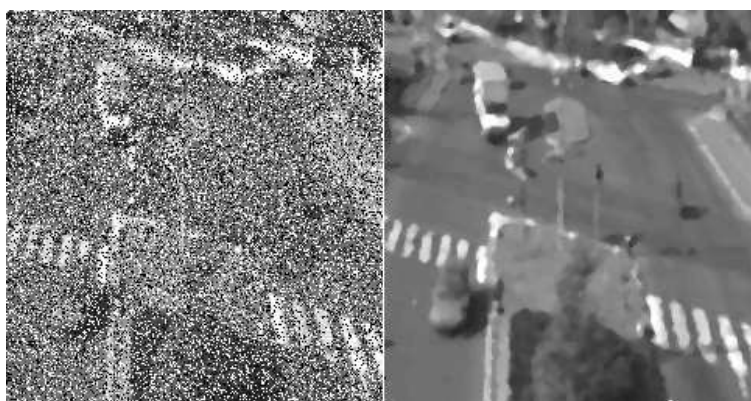
Figure 16.2: Denoising based on a median filter. Left: an image altered on 40% of its pixels with salt and pepper noise. Right: the same image after three iterations of a median filter with a 3 \times 3 square mask.
