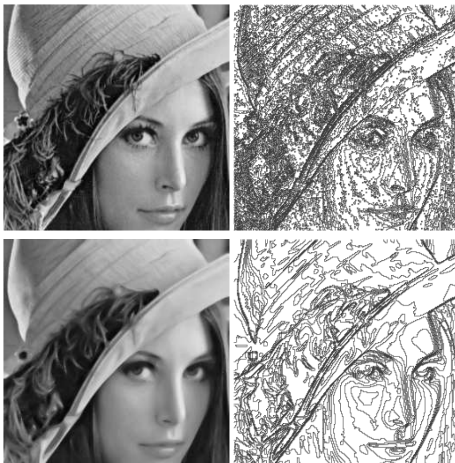
Figure I.20: The affine and morphological scale space (AMSS model). Left to right: original image; level lines of this image (16 levels only); original image smoothed using the AMSS equation; level lines of the third image.
