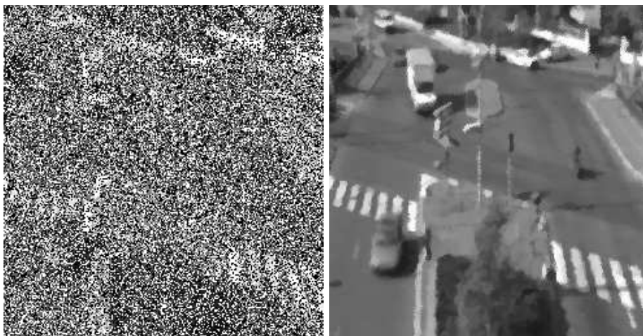
Figure I.3: Denoising. Left: an image with up to 75% of its pixels contaminated by simulated noise. Right: a denoised version by the Vincent-Serra algorithm (area opening).
