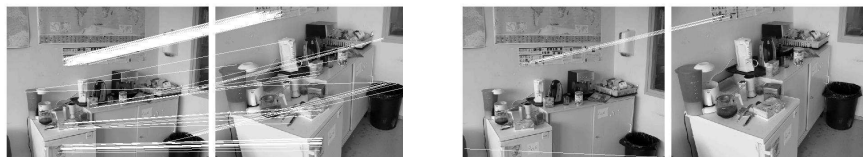
Figure 10.19: Image matching: coffee room. Transition tilt \tau \in [1.5, 3.3] . A-SIFT (shown), SIFT, Harris-Affine, Hessian-Affine, MSER+Corr and MSER+SIFT (shown) find respectively 125, 13, 0, 3, 5 and 2 correct matches. A-SIFT is implemented with K = 1 , which gives one of the very few examples where details in one of the images are so small that K = 2 and K = 3 do not work.
