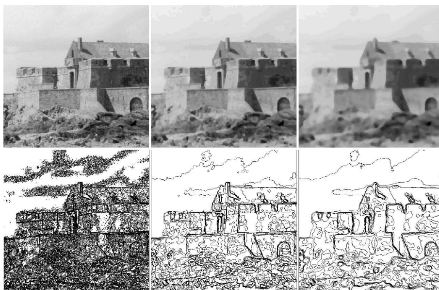
Figure 20.5: Comparing an iterated median filter and a median filter. Top-left: original image. Top-middle: 16 iterations of the median filter with a radius 2, Top-right: one iteration of the same median filter with a radius 8. Below each image are the level-lines for grey levels equal to multiples of 16. This shows that iterating a small size median filter provides more accuracy and less shape mixing than applying a large size median filter. Compare this with the Koenderink–Van Doorn shape smoothing and the Merriman–Bence–Osher iterated filter in Chapter 7, in particular Figures 7.2, 7.1, and 7.4.
