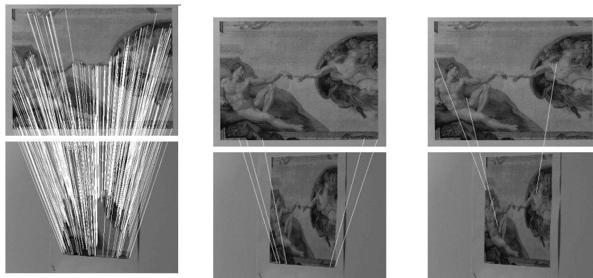
Figure 10.9: Correspondences between long distance snapshots (zoom \times 10 ) at frontal and 65^\circ angle, absolute tilt t = 2.4 . A-SIFT ( K = 3 , shown), SIFT (shown), Harris-Affine (shown), Hessian-Affine, MSER+Corr and MSER+SIFT find respectively 341, 5, 3, 0, 3 and 4 correct matches.
