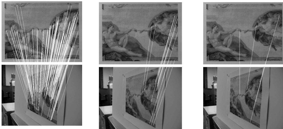
Figure 10.8: Correspondences between the painting images taken from short distance (zoom \times 1 ) at frontal view and at 75^\circ angle. The local absolute tilt varies: t = 4 (middle), t < 4 (right part), t > 4 (left part). A-SIFT ( K = 3 , shown), SIFT (shown), Harris-Affine, Hessian-Affine, MSER+Corr and MSER+SIFT (shown) find respectively 202, 15, 3, 1, 5 and 5 correct matches.
