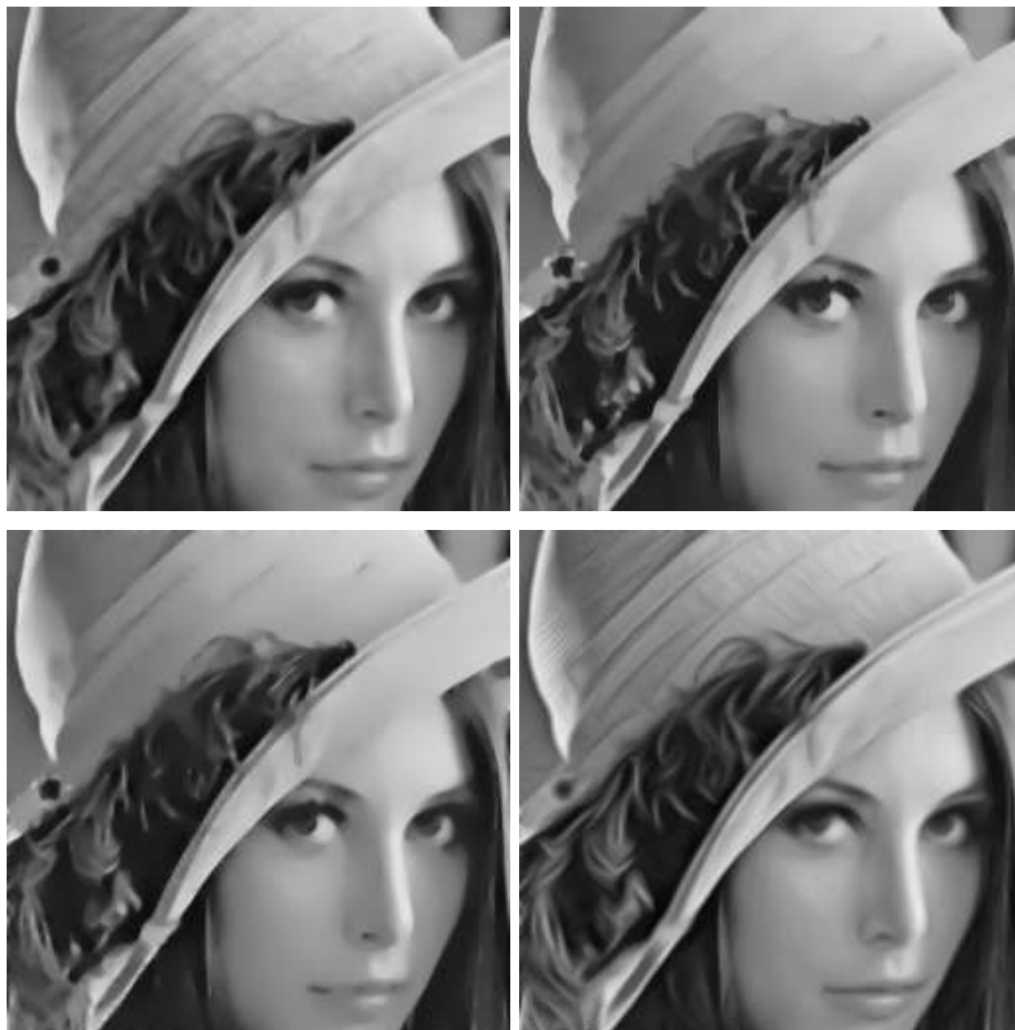
Figure I.13: Diffusion models I. Left to right: Osher, Sethian 1988: the curvature equation; Rudin, Osher, Fatemi 1992: minimization of the image's total variation; Alvarez, Lions, Morel 1992: nonlocal variant of the preceding; Weickert 1994: nonlocal variant of the curvature equation. All of these models diffuse only in the direction orthogonal to the gradient, using a more or less local estimate of this direction. This explains why the results of the filters are so similar. However, the Weickert model captures better the texture direction.
