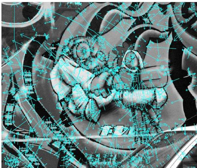
Figure 5.4: SIFT key points. The arrow starting point, length and the orientation signify respectively the key point position, scale, and dominant orientation. These features are covariant to any image similarity.
