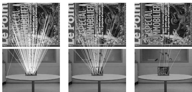
Figure 10.6: Robustness to scale change. A-SIFT (shown), SIFT (shown), Harris-Affine (shown), Hessian-Affine, MSER+Corr and MSER+SIFT find respectively 221, 86, 4, 3, 3 and 4 correct matches. Harris-Affine, Hessian-Affine and MSER are not robust to scale change. A-SIFT is implemented with K = 2 , which means that K = 3 doesn't work.
