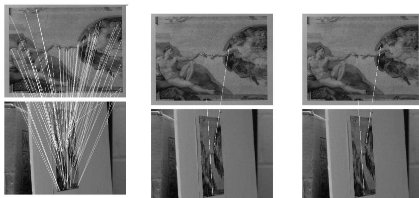
Figure 10.10: Correspondences between long distance views (zoom \times 10 ), frontal view and 80^\circ angle, absolute tilt t = 5.8 . A-SIFT ( K = 3 , shown), SIFT, Harris-Affine, Hessian-Affine, MSER+Corr (shown) and MSER+SIFT (shown) find respectively 75, 1, 1, 0, 2 and 2 correct matches.
