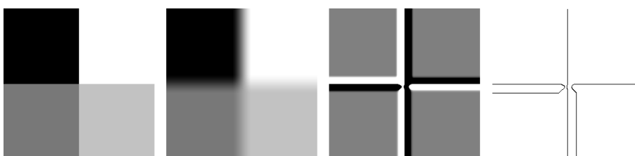
Figure 6.4: Zero-crossings of the Laplacian of a synthetic image. Left to right: the original image; the image linearly smoothed by convolution with a Gaussian; the sign of the Laplacian of the filtered image (the gray color corresponds to values close to 0, black to clear-cut negative values, white to clear-cut positive values); the zero-crossings of the Laplacian. This experiment clearly shows a drawback of the Laplacian as edge detector.
