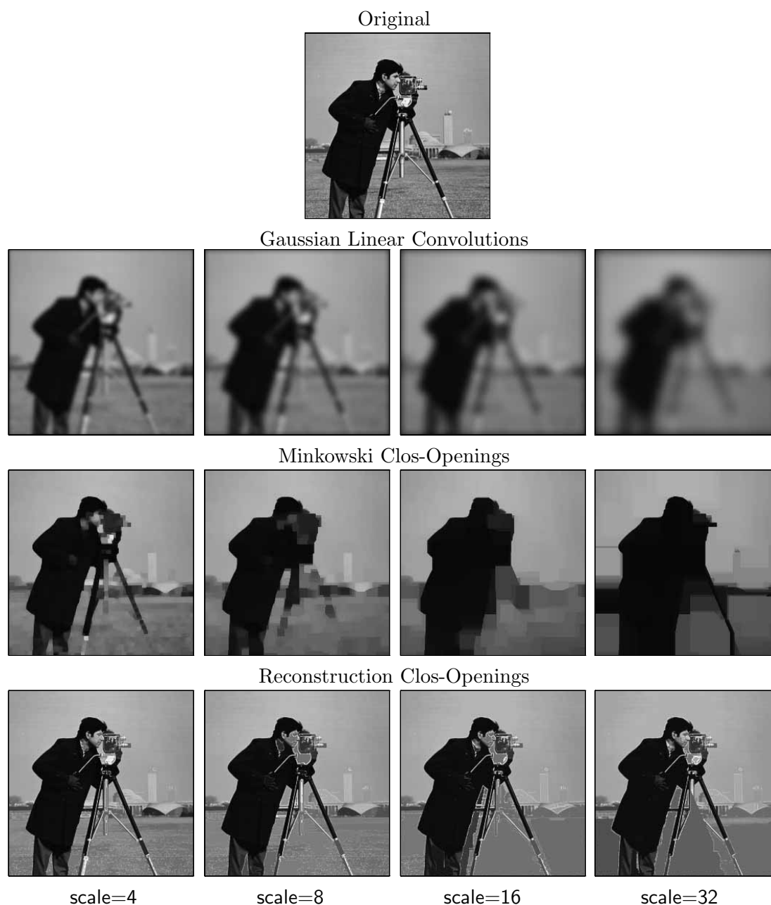
Figure 1: Linear and morphological multiscale image smoothers. (The scale parameter was defined as: the variance of the Gaussians for linear convolutions; the radius of the structuring element for clos-openings; the scale of the marker for the reconstruction filters.)
