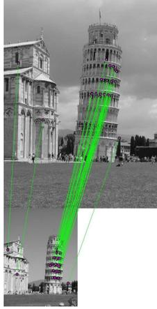
Figure 5.1: A result of the SIFT method, using an outliers elimination method [219]. Pairs of matching points are connected by segments.
