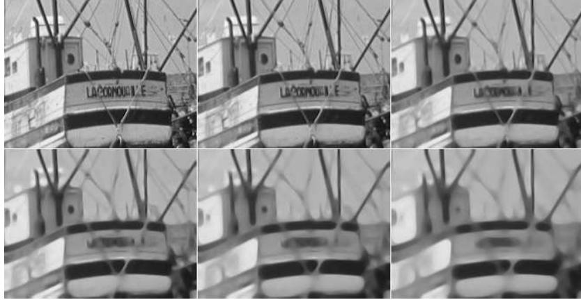
Figure 13.3: Curvature motion finite difference scheme and scale calibration. Image filtered by curvature motion at scales 1, 2, 3, 4, 5. In order to give a sound numerical meaning to the scale, a calibration of the numerical scales (number of iterations) is made in such a way that a disk with radius t shrinks to a point at scale t .
