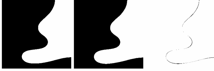
Figure 20.2: Comparing an iterated median filter with a curvature motion. Numerically, the iterated median filter and the curvature motion must be very close, at least when the curvatures of the level lines are not too small. Indeed, the iterated median filter converges towards the curvature motion. Left: the initial shape of Figure 20.1 has been smoothed by a finite difference scheme of the curvature motion; middle: smoothing with a median filter at the same scale; right: difference between left and middle images. The difference is no greater than the width of one pixel. To have a rigorous comparison, scales have been calibrated by ensuring that for both schemes and all r a circle with radius r vanishes at scale r
