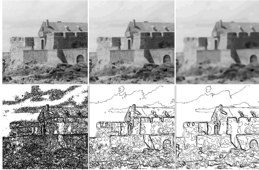
Figure 14.5: Comparing an iterated median filter and a median filter. Top-left: original image. Top-middle: 16 iterations of the median filter with a radius 2, Top-right: one iteration of the same median filter with a radius 8. Below each image are the level-lines for grey levels equal to multiples of 16. This shows that iterating a small size median filter provides more accuracy and less shape mixing than applying a large size median filter. Compare this with the Koenderink–Van Doorn shape smoothing and the Merriman–Bence–Osher iterated filter in Chapter 4, in particular Figures 4.2, 4.1, and 4.4.
