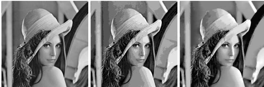
Figure I.15: Diffusion models III. Left to right: original image; quantized image (only 10 levels are kept - 3.32 bits/pixel); the quantized image reinterpolated using the Caselles–Sbert algorithm 1998. They apply a diffusion on the quantized image with values on the remaining level lines taken as boundary conditions.
