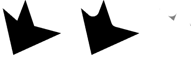
Figure 9.4: Closing of a set as a curvature threshold from below. Left to right: A set X ; its closing by a ball of radius 20; the difference set. The closing of X is just the opening of X^c . It can be viewed as a threshold from below of the curvature of the set boundary.
