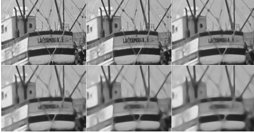
Figure 13.4: Curvature motion finite difference scheme applied on each level set separately, at scales 1, 2, 3, 4, 5. The processed image is then reconstructed by the threshold superposition principle. In contrast with the same scheme directly applied on the image, this scheme yields a fully contrast invariant smoothing. However, a comparison with Figure 13.3 shows that the resulting images are very close to each other. This shows that the contrast invariance is almost achieved when applying the finite difference scheme directly on the image. The experiment makes sense if the original image is of good quality, that is relatively smooth and with no strong oscillations. In that case, it can be considered as a distance function to each one of its own level sets. As we shall see in Figure 13.6, if the initial image is noisy, the difference between both methods can be huge.
