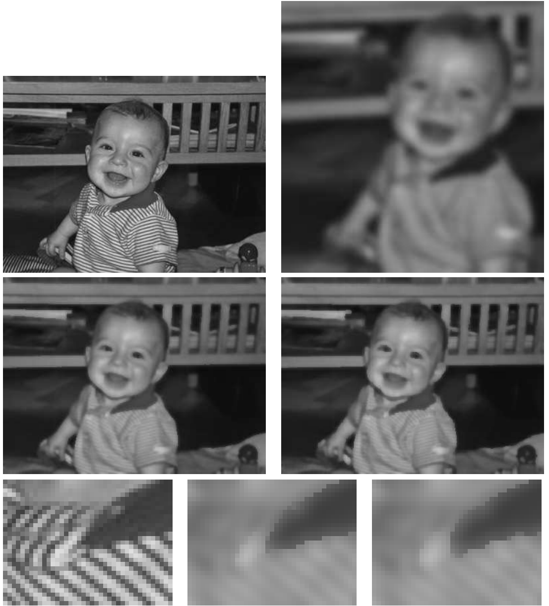
Figure 23.1: Shock Filter implemented by using non flat morphological filters. Top, left :original image, right: blurred image using Heat Equation, Middle-left: two iterations of the kramer filter, Middle-right: two iterations of the Rudin-Osher filter. The scale parameter is chosen such that the parabola passes the range of the image at a distance of 6 pixels. Down: zoom version of a detail, left: original image, middle: kramer filter, right: Rudin-Osher filter. We see a tendency of this last to smooth shapes toward circles.
