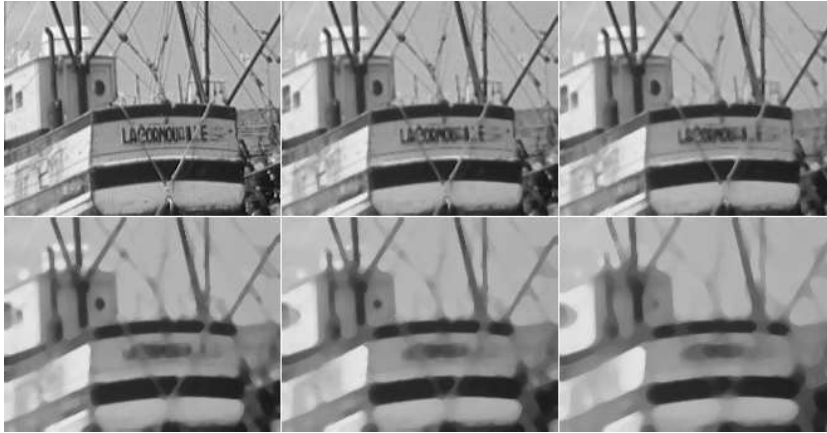
Figure 13.5: Iterated median filter with normalized scales 1, 2, 3, 4, 5. The scale normalization permits to compare very different schemes on the same images. Compare with Figure 13.4. The striking similarity of the results anticipates Theorem 14.7, according to which the application of the median filter is equivalent to a mean curvature motion.
