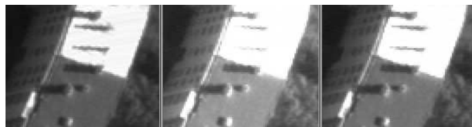
Figure 6.4: Extracts from the stereo pair shown on Figure 6.3. From left to right: in the original image, in the specified one, in the original image after midway equalization. Notice that no detail is lost in the midway image, in contrast with the middle image.
