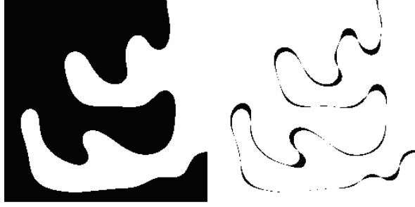
Figure 14.2: Median filter and the curvature of level lines. Smoothing with a median filter is related to the curvature of the level lines. Left: image of a simple shape. Right: difference of this image with itself after it has been smoothed by one iteration of the median filter. We see, in black, the points which have changed. The width of the difference is proportional to the curvature, as indicated by Theorem 14.7.
