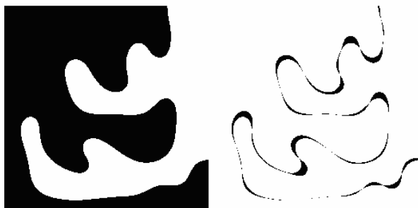
Figure 13.2: Median filter and the curvature of level lines. Smoothing with a median filter is related to the curvature of the level lines. Left: image of a simple shape. Right: difference of this image with itself after it has been smoothed by one iteration of the median filter. We see, in black, the points which have changed. The width of the difference is proportional to the curvature, as indicated by Theorem 13.7.
