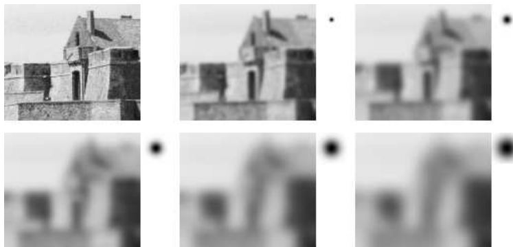
Figure 1.3: Convolution with Gaussian kernels (heat equation). Displayed from top-left to bottom-right are the original image and the results of convolutions with Gaussians of increasing variance. A grey level representation of the convolution kernel is put on the right of each convolved image to give an idea of the size of the involved neighborhood.
