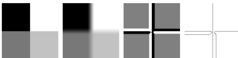
Figure 3.4: Zero-crossings of the Laplacian of a synthetic image. Left to right: the original image; the image linearly smoothed by convolution with a Gaussian; the sign of the Laplacian of the filtered image (the gray color corresponds to values close to 0, black to clear-cut negative values, white to clear-cut positive values); the zero-crossings of the Laplacian. This experiment clearly shows a drawback of the Laplacian as edge detector.
