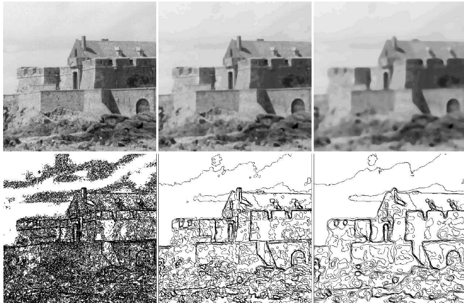
Figure 13.5: Comparing an iterated median filter and a median filter. Top-left: original image. Top-middle: 16 iterations of the median filter with a radius 2, Top-right: one iteration of the same median filter with a radius 8. Below each image are the level-lines for grey levels equal to multiples of 16. This shows that iterating a small size median filter provides more accuracy and less shape mixing than applying a large size median filter. Compare this with the Koenderink–Van Doorn shape smoothing and the Merriman–Bence–Osher iterated filter in Chapter 4, in particular Figures 4.2, 4.1, and 4.4.
