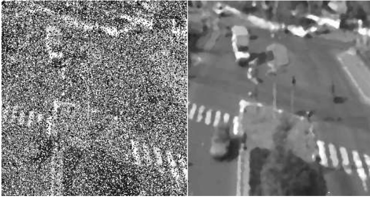
Figure 10.2: Denoising based on a median filter. Left: an image altered on 40% of its pixels with salt and pepper noise. Right: the same image after three iterations of a median filter with a 3 \times 3 square mask.
