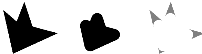
Figure 9.3: Opening of a set as curvature threshold from above. Left to right: A set X ; its opening by a ball of radius 20; the difference set. This opening transforms X into the union of all balls of radius 20 contained in it. The resulting operation can be understood as a threshold from above of the curvature of the set boundary.
