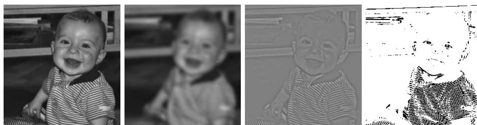
Figure I.10: The Laplacian pyramid of Burt and Adelson. Left to right: the original image; the image blurred by Gaussian convolution; the difference between the original image and the blurred version, which approximates the Laplacian of the original image; the points where this Laplacian image is large.
