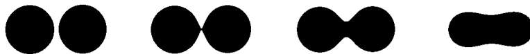
Figure 4.1: Nonlocal interactions in the dynamic shape method. Left to right: Two close disks interact as the scale increases. This creates a new, qualitatively different, shape. The change of topology, at the scale where the two disks merge into one shape, also entails the appearance of a singularity (a cusp) on the shape(s) boundaries.
