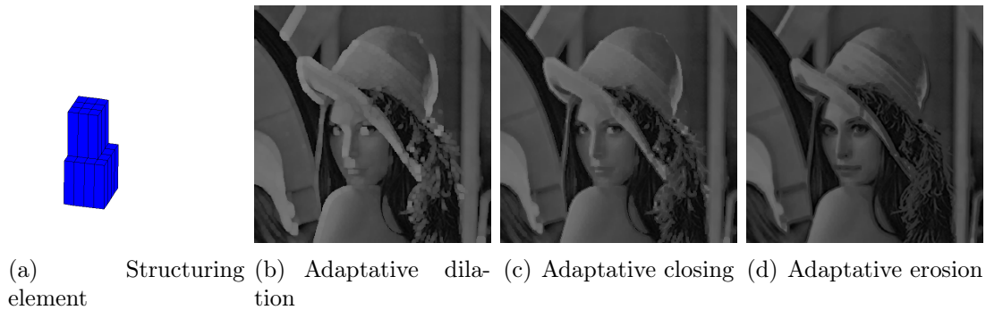
Figure 4.2: Adaptive morphology with a structuring element maximal in the middle
