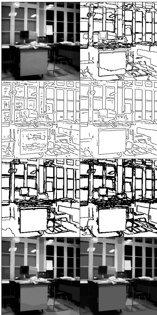
Fig. 9.11. First row: left: original image; right: boundaries obtained with the Mumford-Shah model (1000 regions). Second row: edges obtained with Canny-Deriche edge detector for two different threshold values (2 and 15). Third row: meaningful edges (left) and meaningful boundaries (right) obtained with \varepsilon = 1 . Fourth row: reconstruction with the Mumford-Shah model (left) and with the set of meaningful boundaries (right). This last reconstruction is easily performed by the following algorithm: Attribute to each pixel x the level of the smallest (for inclusion) meaningful level line surrounding x (see [Mon00]).
