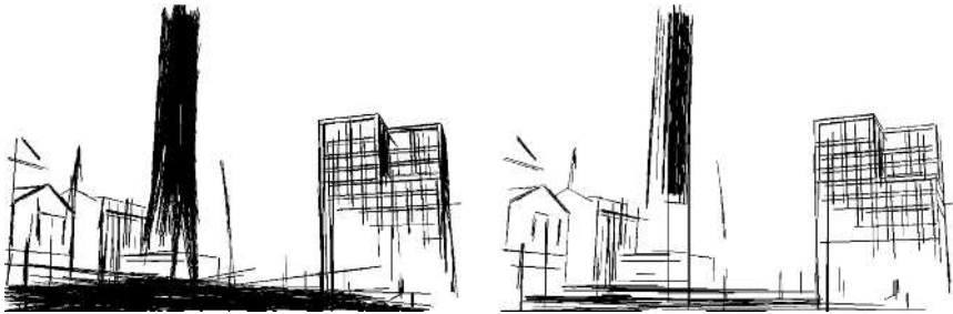
Fig. 6.2 Parallelism against alignment. Top: original Brown image. Bottom-left: maximal meaningful alignments as defined in Section 6.3. Here, since many parallel alignments are present, secondary parasite slanted alignments are also found. Bottom-right: alignments finally obtained by the exclusion principle, explained in Section 6.2, which eliminates the remaining spurious alignments. The experiment proves that maximal meaningfulness by itself cannot remove the slanted alignment detections that arise from bundles of parallel alignments. The more general exclusion principle is therefore necessary.
