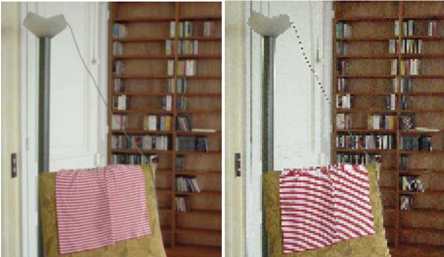
Fig. 1.2 On the left, a well-sampled image according to the Shannon-Nyquist principle. The relations between sample distances and the Fourier spectrum content of the image are in conformity with Principle 1 and Algorithm 1. If these conditions are not respected, the image may undergo severe distortions, as shown on the right.
