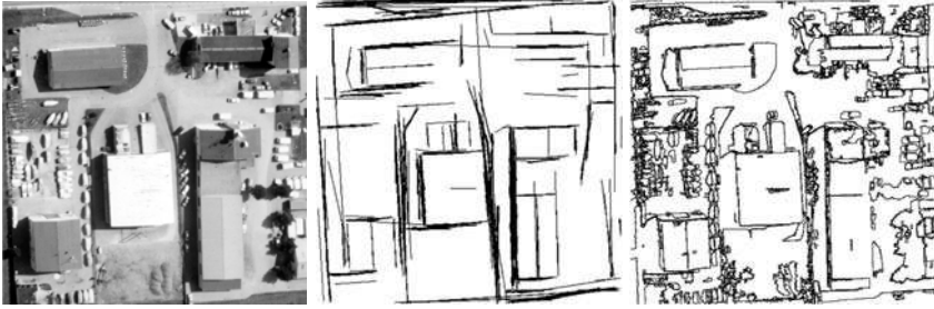
Fig. 1.4 Left: original aerial view (source: INRIA); middle: maximal meaningful alignments; right: maximal meaningful boundaries.
