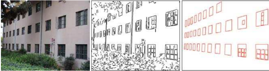
Fig. 15.2 Example of results of Han and Zhu. From left to right: input image; edge map; rectangles detected and grouped. (Figures courtesy of S.C. Zhu.)
