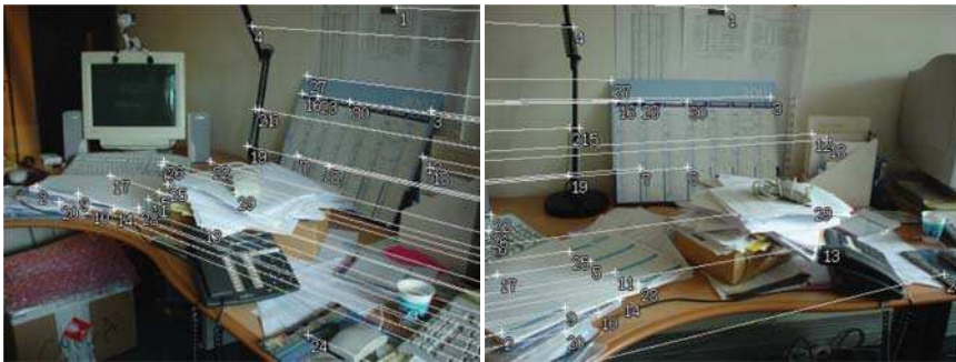
Fig. 12.11 The second stereo pair with 70 point matches (only 30 are shown here for clarity). The epipolar geometry is recovered in no time and yields \text{Log } \alpha = -1.92 and \text{Log } \varepsilon = -110 .
