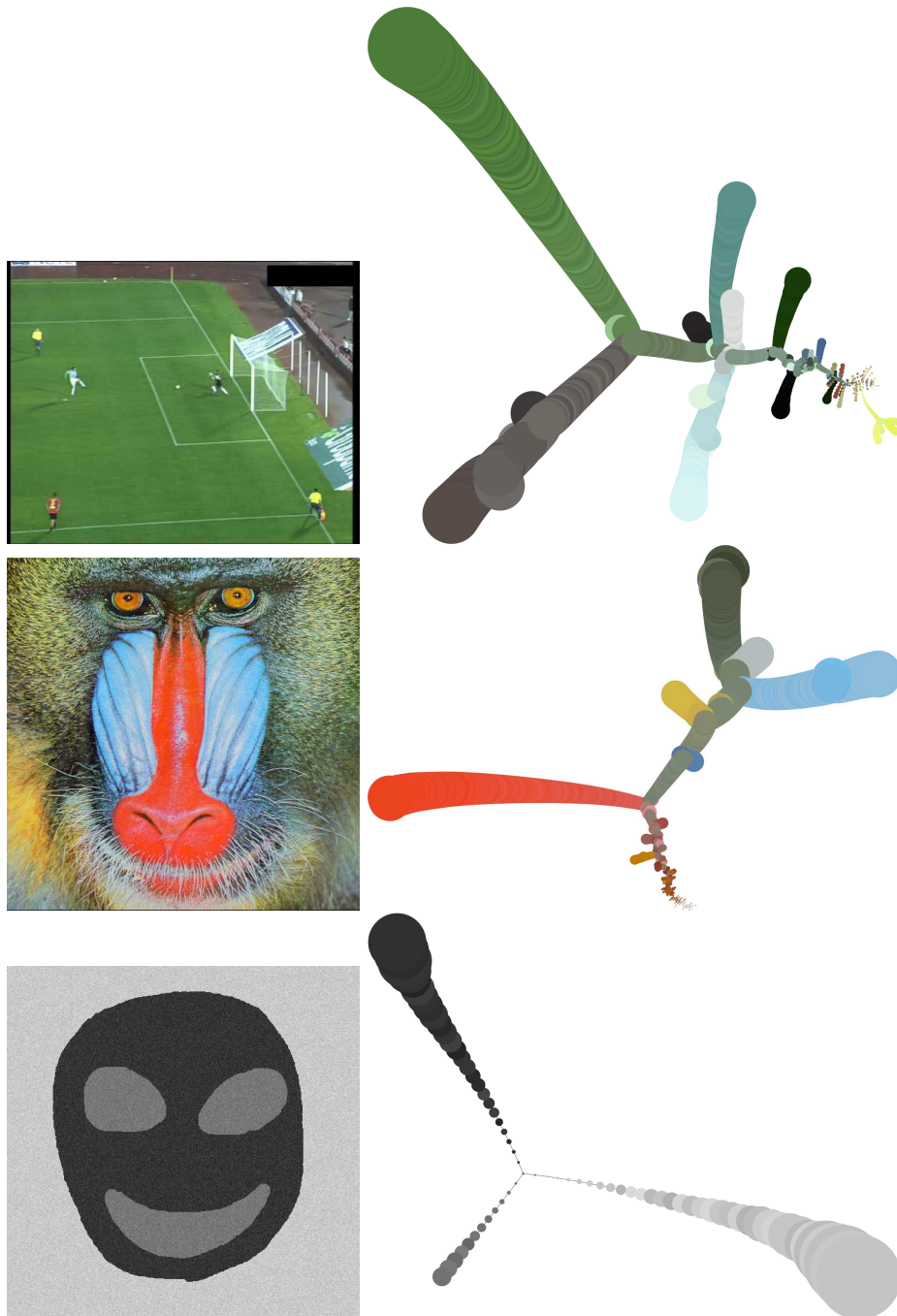
Figure 5.12: The tree of shapes of color histograms, as visualized by a standard graph-drawing program ( neato ). These pictures are the graphs of the tree of shapes, suitably decorated . Each node is a coloured to the mean color of the corresponding region on colour space, and the radius of the disc is the (logarithm of) the pixel count inside that region.
