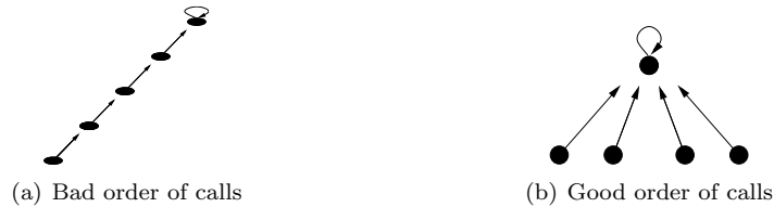
Figure 4.11: The tree structure depends on the order of the calls to the set-union function.
