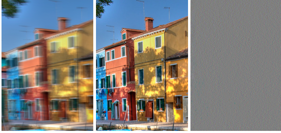
Figure A.18 – M.I.P. code : observed image (left). The blur interval length is equal to 52 pixels here. Reconstructed image ( RMSE = 2.11 ) (middle). Residual noise (difference between ground truth and reconstructed, dynamic normalized on [0, 255] by an affine contrast change).
