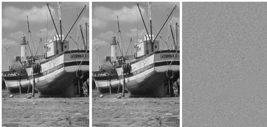
Figure A.8 – Snapshot : observed image (left). The blur interval length is equal to 1 pixel here. Reconstructed image ( RMSE = 1.47 ) (middle). Residual noise (difference between ground truth and reconstructed, dynamic normalized on [0, 255] by an affine contrast change).
