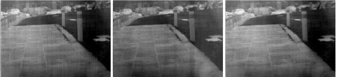
Figure A.9 – On the left : a real raw image of an outdoor scene taken by an infrared camera. Middle : the total variation based method. Notice the artifacts created below the poles. On the right the proposed method (we deactivate the DCT denoising to provide a fair comparison).
