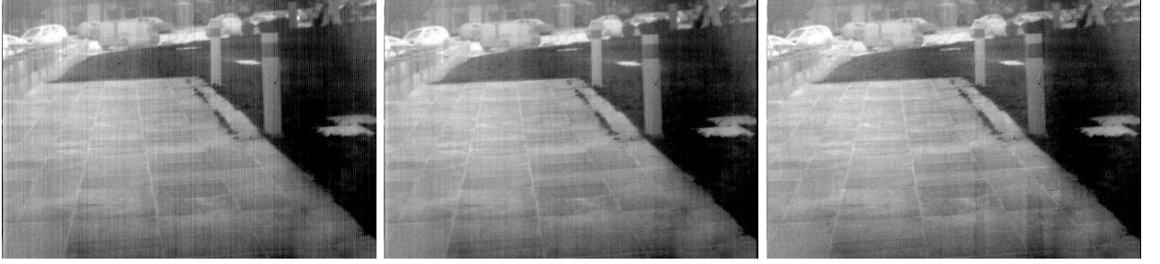
Figure A.5 – On the left : a real raw image produced by an infrared camera. Middle : the result of the algorithm with the parameter s = 1 . On the right with s = 7.5 . For example, focusing on a zone in the middle of the image the image with s = 7.5 is nicer but, the zone below poles is bad. On the other hand in the image processed with s = 1 the zone in the middle is still corrupted by the non uniformity . Thus, a fixed s parameter for the whole image will not lead to the best quality possible everywhere.
